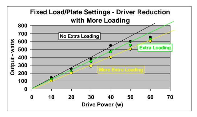
Figure 4. Effect of driver power reduction with fixed Plate/Load settings for 3 levels of loading.
