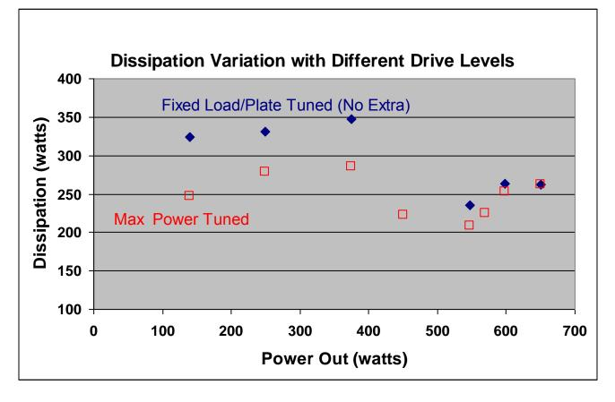
Figure 5. Variation of dissipation with drive power reduction.
