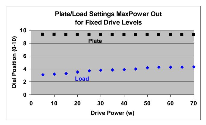
Figure 2. Plate and Load amp setting for max power out for the same conditions in the first figure.
